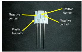
The core of the InstaLoad technology is the individual battery contacts assembly. The relationship between the battery terminals and the InstaLoad battery contacts is shown in the figure below. At one end of the battery, the battery interfaces with either the positive contacts (light gray) or the negative contacts (black). The battery interfaces with the opposite contact at its other end. When coupled with PCB traces, proper power polarity is automatically delivered to the device.
